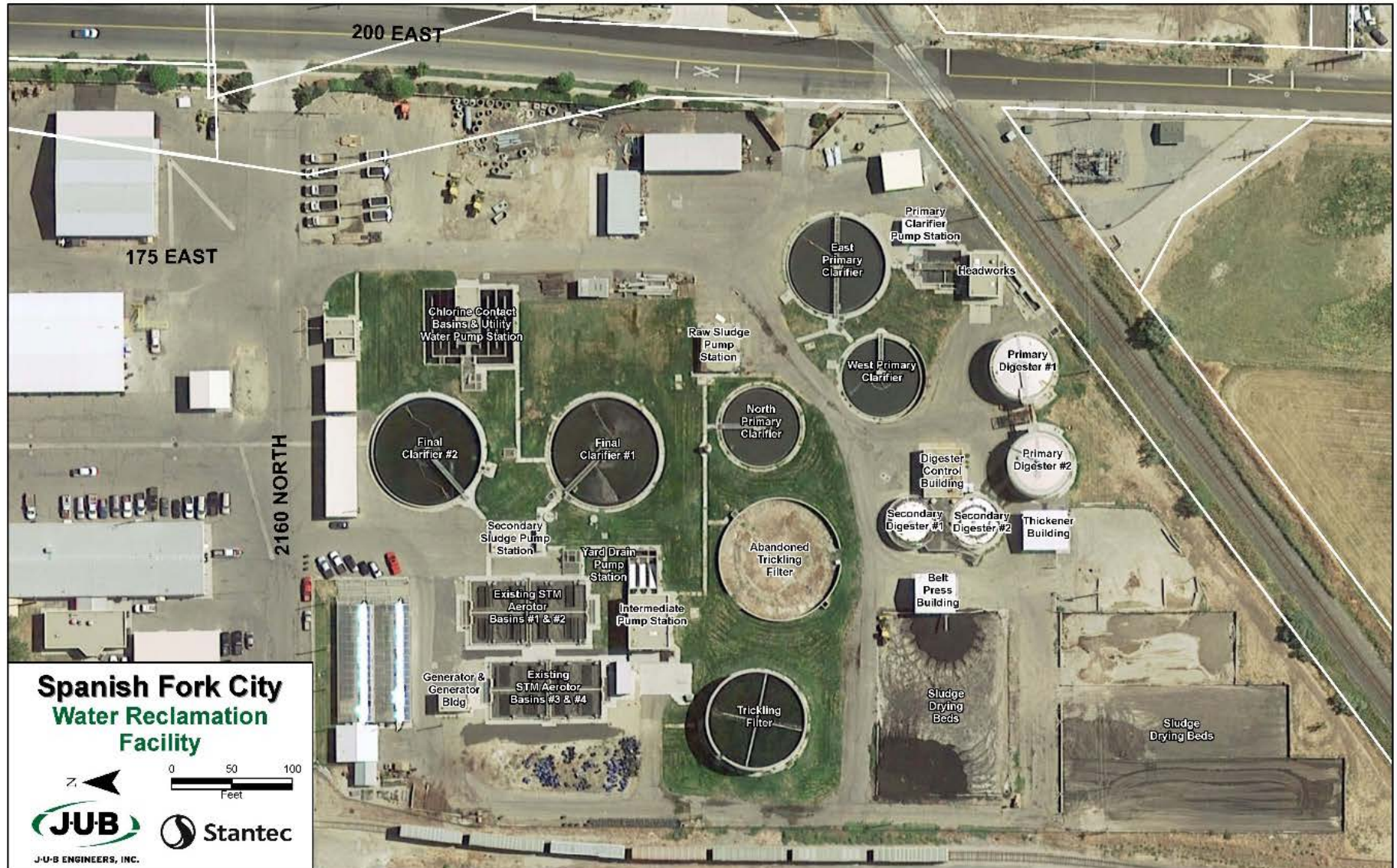
Figure 2-1: Spanish Fork WWTP Existing Site Layout
